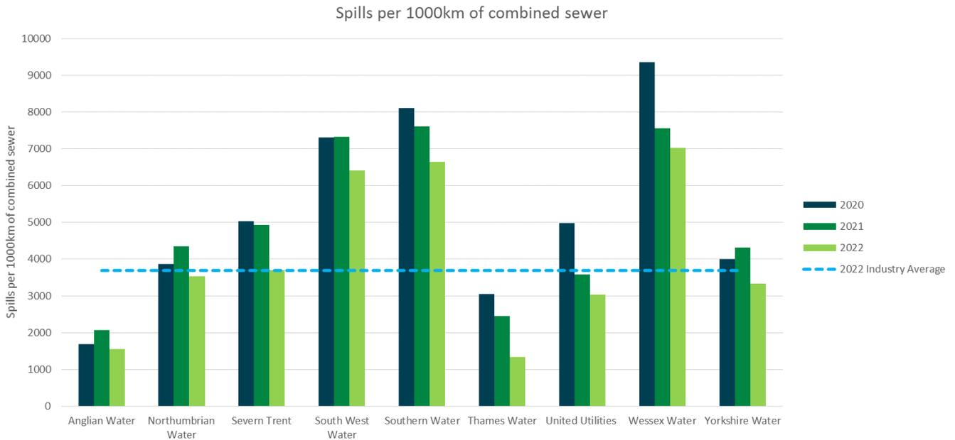
Source: UUW analysis of industry EDM data<sup>4</sup> normalised by APR datashare
